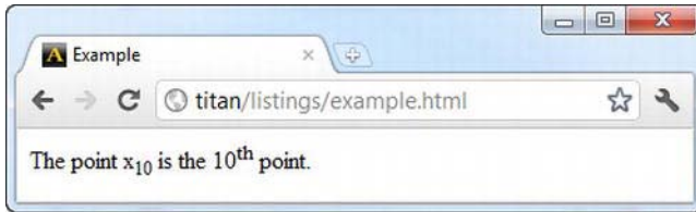
Figure 8-9. Using the sub and sup elements
