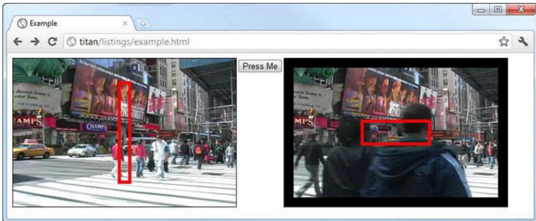
Figure 35-22. Using one canvas as the source for the drawImage method on another canvas
