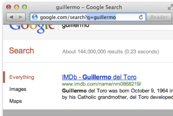
Figure 7-14: The highlighted part in the URL when a search is performed is q=<search term> .
