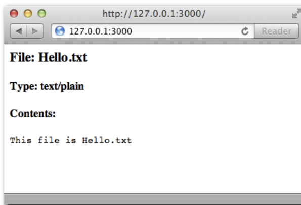
Figure 8-9: The contents of sample file Hello.txt shown through the browser after the successful upload
