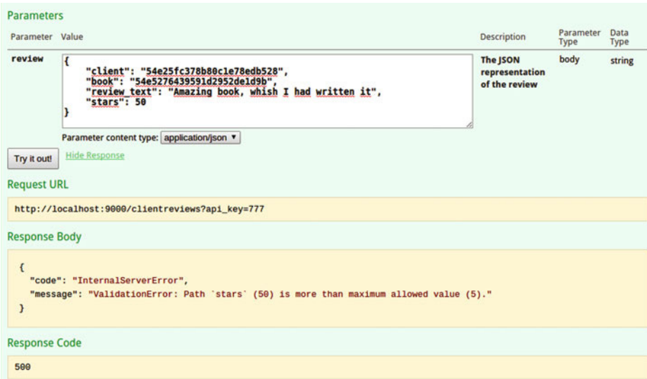
Figure 7-2. An error when trying to save an invalid value in a validated model
