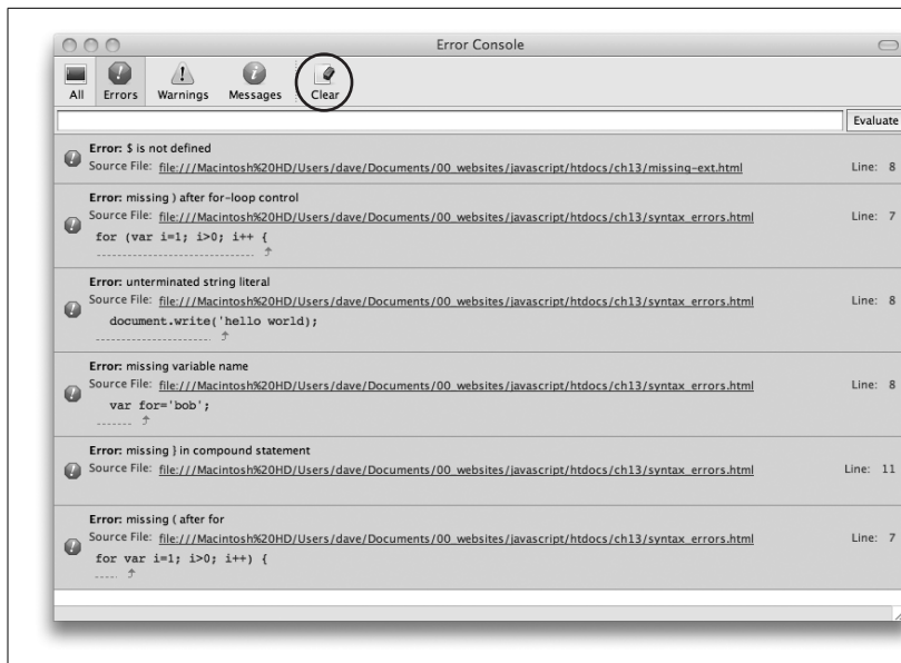
Figure 13-1: Firefox's Error Console lists all JavaScript errors that the browser encounters. You can display the console by choosing Tools → Error Console. Since the console lists the errors it has encountered on all pages, you'll want to frequently erase the list by clicking the Clear button (circled).
