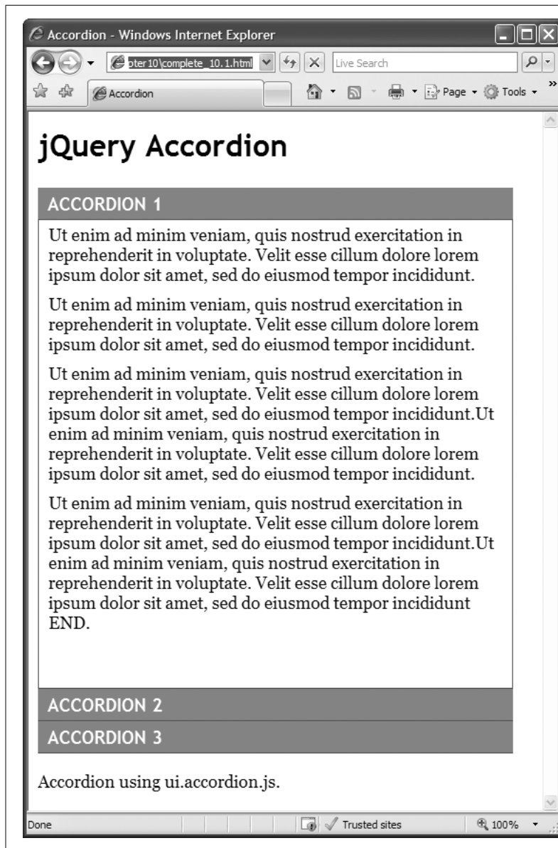
Figure 10-2: Adding an accordion to a Web page requires nothing more than some basic HTML, jQuery, the Accordion plug-in, and a few lines of code.
