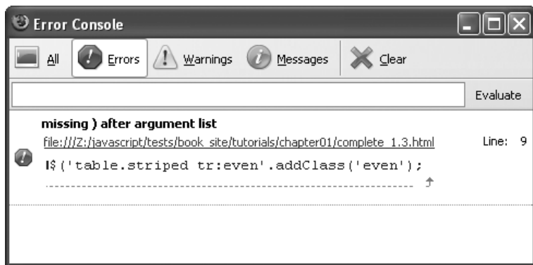
Figure 1-6: Firefox's JavaScript console identifies errors in your programs. The console keeps a list of errors for previous pages as well, so pretty soon the list can get very long. Just click the Clear button to erase all the errors listed in the console.
