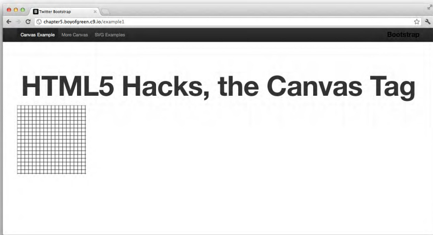
Figure 4-1. The 200 × 200 <canvas> tag with grid markers every tenth point on both the x- and y-axes
