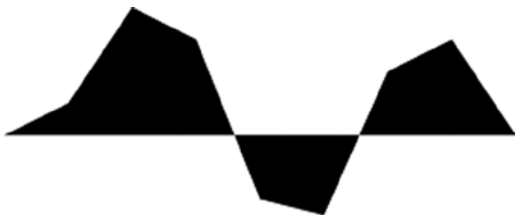
Figure 20-2. The default behavior of an SVG path element is to draw filled areas
