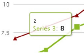
Figure 18-2. By default, a tooltip reports the x and y values of the point and the name of the series to which it belongs
