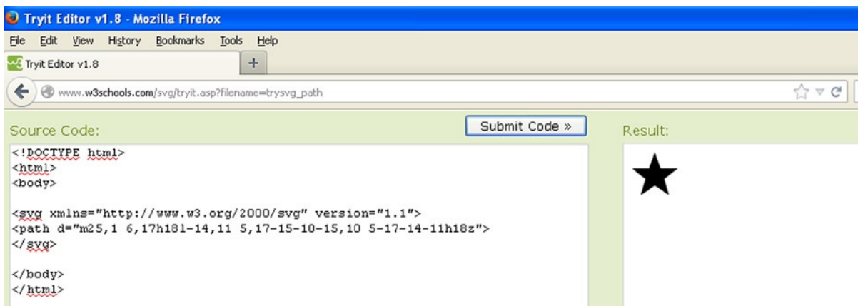
Figure 24-4. Tryit is a useful tool to preview SVG symbols in real time inserting the path
